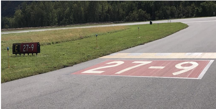
Surface Painted Holding Position Sign on the taxiway at the runway holding position marking
